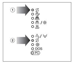
When the salt reservoir is empty the S indicator light <sup>(2)</sup> comes on. The reservoir should be refilled with dishwasher salt for reactivation.
